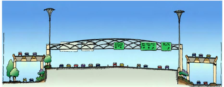
is functionally sound and provides a visual association with the type of bridge structures often used to span creeks and rivers. If implemented, this simple strategy would lend another aspect of interest while still serving the primary functional needs of the project. Sign columns could potentially be of concrete construction if space permits. If so, this would enable the columns to incorporate detailing from other structural members such as bridge and retaining wall columns.
