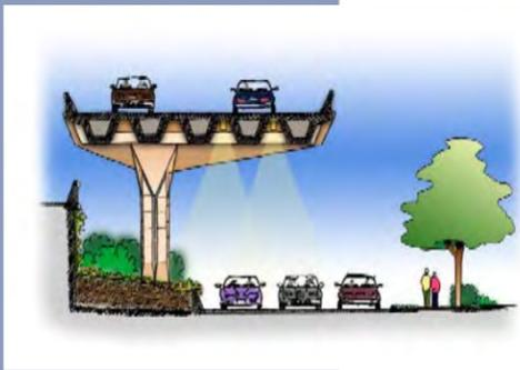
Columns supporting the bridge beams and deck should be designed to relate to other structural surface finishes in a coordinated fashion. In general, a twin column relief is recommended with details such as the column base and/or cap details varying by project segment. This strategy acknowledges the inherent consistency of certain bridge components through all areas of the project with minor details varying in accordance with the context sensitive design strategy for the overall project.
