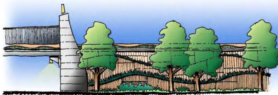
walls along each side of the new facility. In essence, these walls will replace the existing sloped shoulders to accommodate the upgraded facility. This will require the removal of most turf areas and trees that currently exist between the freeway mainlanes and frontage roads along IH 35E.
